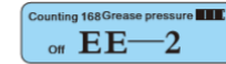
s Alarm due to insufficient filling (It has no influence on system operation. Fault will be automatically cleared at the time of need normal operation)
