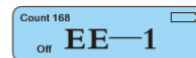
r Alarm due to lack of grease (Alarm sends and the machine will be shut down after 6 consecutive operations, the alarm will be automatically acknowledged after the tank is fully filled)
