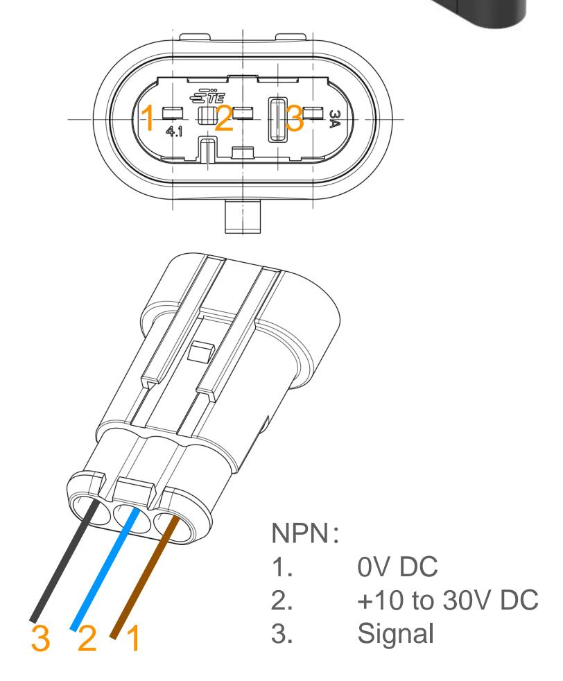
Dia. 18.2 Divider Monitoring Sensor Wiring Connection
