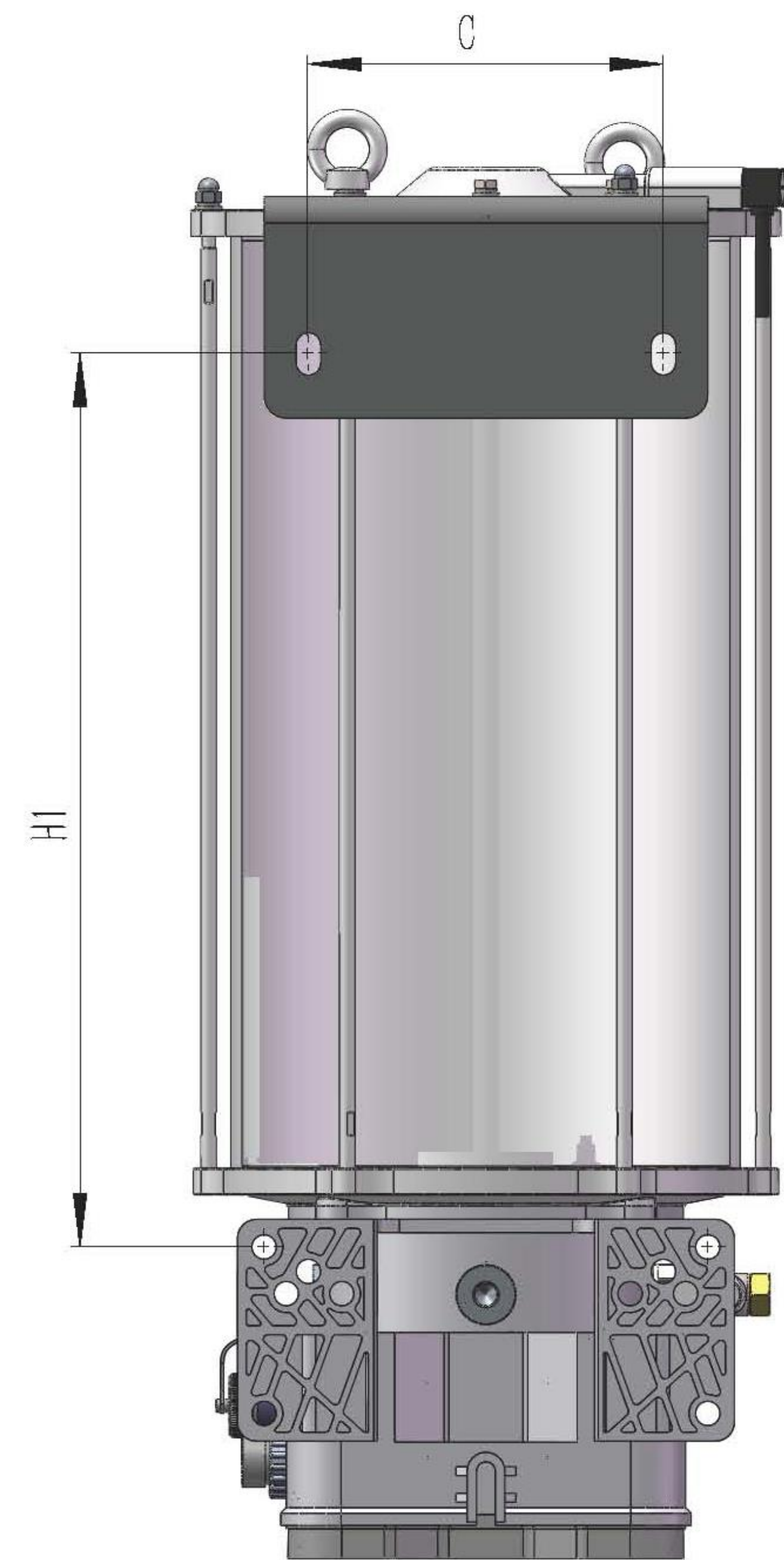
Dia. 11.3 Mounting dimensions for ALPB pump (Stirring paddle type) on Top for Pump 15L and 20L
