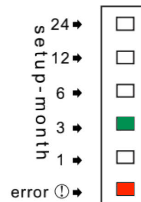
Dia. 9.2 Overloading warning (blockage)
