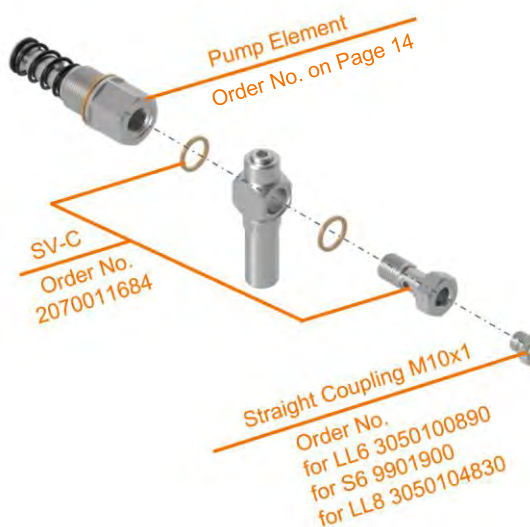
Dia. 16.2 Explosion for SV-C with PE + Straight Coupling
