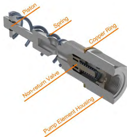
Dia. 14.2 Pump Element structure
