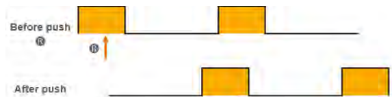
Dia. 24.5 Cycle changing when push Ⓜ during Lube time
