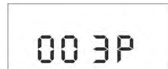
Dia. 23.6 Setting of 3P - Lube Time in Minute
