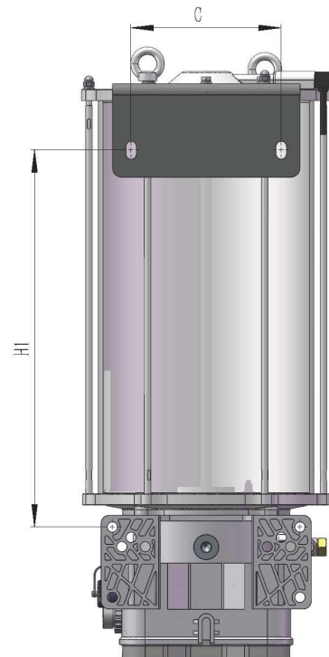
Dia. 19.3 Mounting dimensions for ALPB pump (Stirring paddle type) on Top for Pump 15L and 20L
