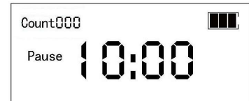
Dia. 23.2 "Pause time" display after first power connection
