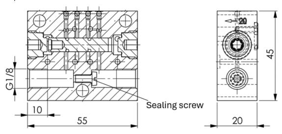
In this way, the dosage quantities of the individual divider elements can always be dosed appropriately for each lubrication point.
