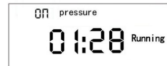
Fig. 3 Display Lube time 3P counting up
