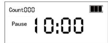
Fig. 2 Pause time display after first power connection
