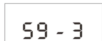
Fig. 7 Setting 3P Lube time in second
