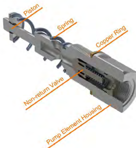
Dia. 14.2 Pump Element structure
