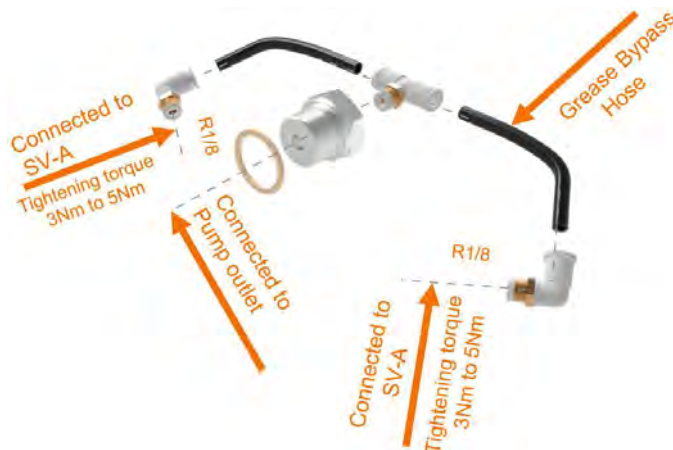
Dia. 18.6 Explosion of Dual Bypass
