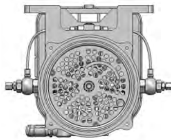
Dia. 18.3 Pump with 2 safety valve type A + Dual Bypass
