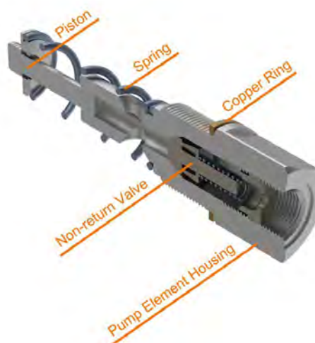
Dia. 14.2 Pump Element structure
