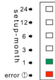
Dia. 9.1 No motor pulse warning (low battery)
