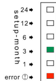
Dia. 9.2 Overloading warning (blockage)
